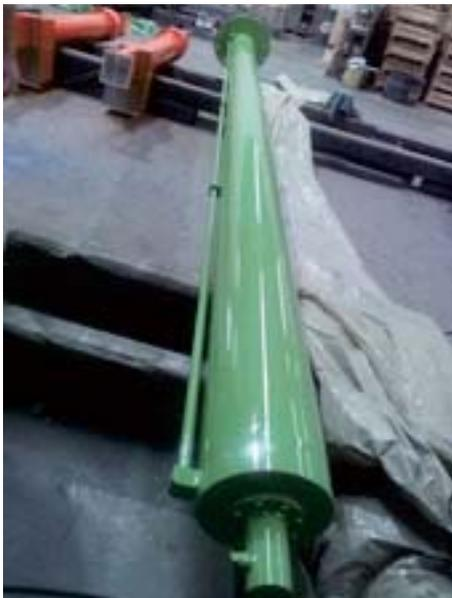
6550mm hydraulic cylinder uses 19 series
