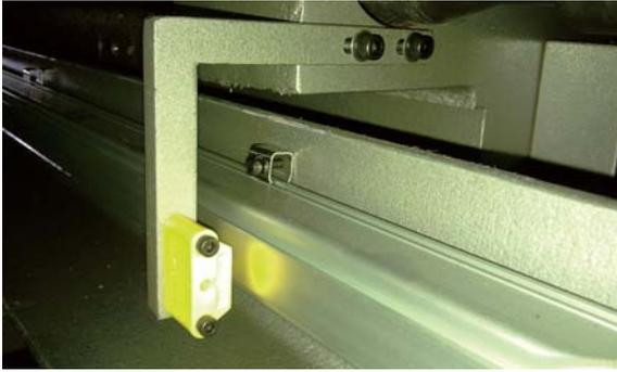
Installation of floating magnet is very simple. Compared to captive magnet, floating magnet can truly demonstrate the advantage of non-contact sensing and eliminate the wear of captive magnet socket.
