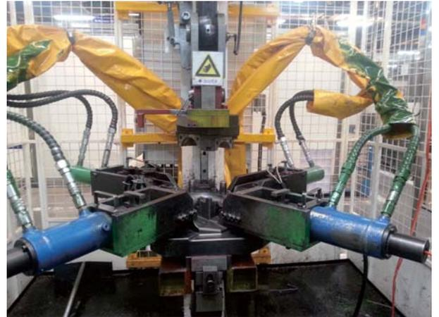
Automotive exhaust pipe bending machine used Germanjet 17 series
