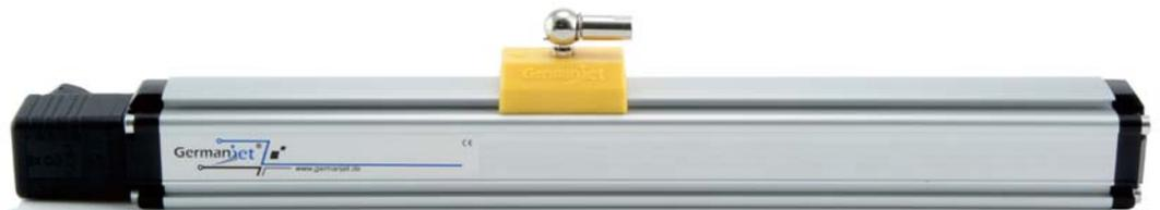
The fundamental principle of the magnetostrictive transducer is by analyzing the feedback sonic wave induced by an interaction of two magnetic fields. The first magnetic field is produced by the moveable magnetic cursor which attached at the moving component of a machine. The second field is generated by the pulse initiator. After the two magnetic fields interact, a sonic wave is induced and detected by the sonic wave analyzer.
